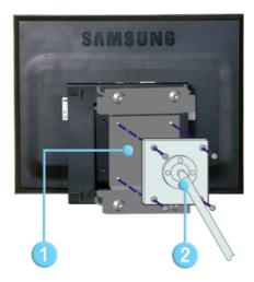
Squeeze the folded monitor stand into the VESA mounting bracket. Then fasten it using the four supplied nuts with the monitor, mounting pad and VESA mounting bracket aligned.
